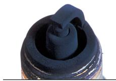
**Carbon fouling** Appearance: Dry, soft black carbon on the insulator and electrodes. Results:
