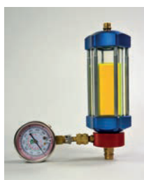
Refrigerant R134a mixed with - DENSO ND8 (PAG46) - UV Leak Dye
