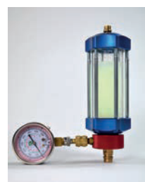
Refrigerant R134a mixed with - DENSO ND8 (PAG46) - Universal Oil (PAO68)
