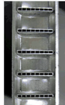
Cross-section through the condenser tubes
