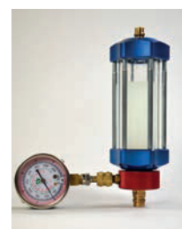
Refrigerant R134a mixed with - DENSO ND8 (PAG46) - DENSO ND11 (POE-Insulating Oil)
