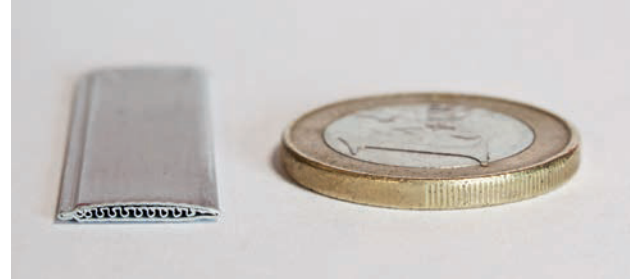
A comparison with a 1 euro coin illustrates the size of the tiny condenser cooling capillary.
