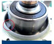
Fusing point resin crack
