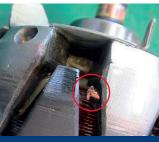
Rotor coil wire breakage
