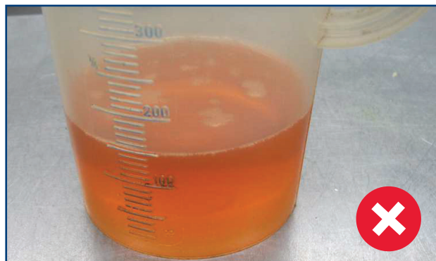
ND-oil: saturated with moisture
