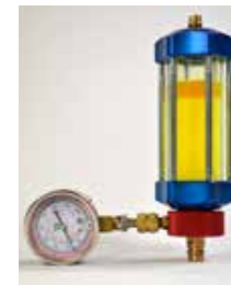
Refrigerant R134a mixed with - DENSO ND8 (PAG46) - UV Leak Dye - Universal Oil (PAO68) R134a, PAG46 Oil and UV leak dye are mixed. PAO68 Oil floats on top. Slight milky/coloured appearance.
