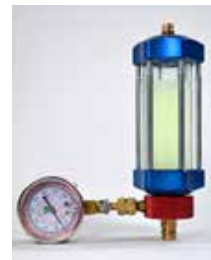
Refrigerant R134a mixed with - DENSO ND8 (PAG46) - Universal Oil (PAO68) R134a and PAG46 Oil are mixed. PAO68 Oil floats on top. Slight milky appearance.
