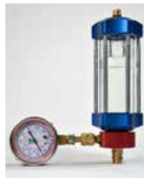
Refrigerant R134a mixed with - Universal Oil (PAO68) Clear liquids that do not mix with each other
