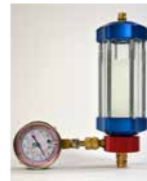
Refrigerant R134a mixed with - DENSO ND8 (PAG46) - DENSO ND11 (POE-Insulating Oil) All liquids are mixed with each other. Slight milky appearance.
