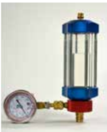
Refrigerant R134a mixed with - DENSO ND8 (PAG46) Clear mixture with slight streaks
